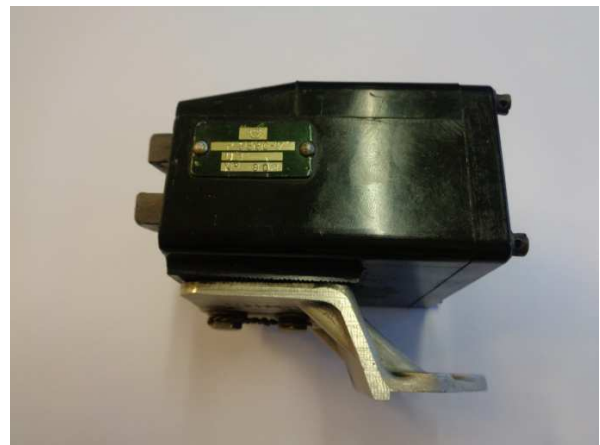
Fig.2 Brush block assembly P/N:P3560-7
